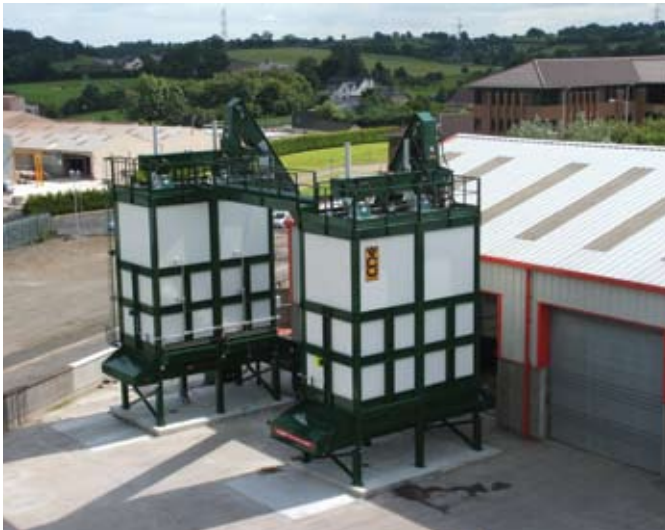
Magherafelt District Council, Northern Ireland, process co-mingled food and green waste in its VCU™ system
